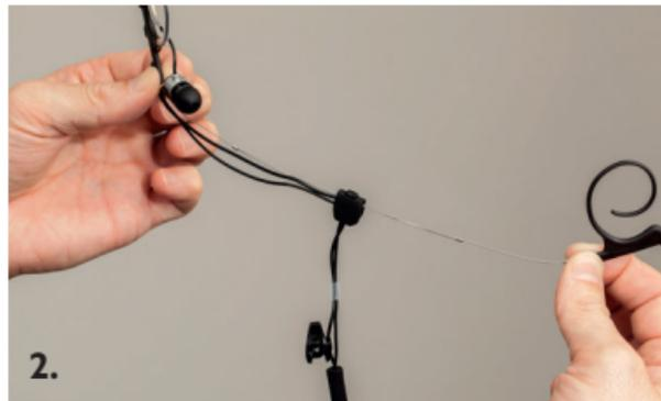
1. Hold cable lock and draw cables to create excess:
